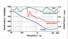
Fig. 2—On-axis phase response, group delay, and waveform phase.
