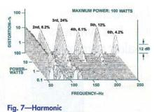
distortion for E<sub>1</sub> (41.2 Hz).
